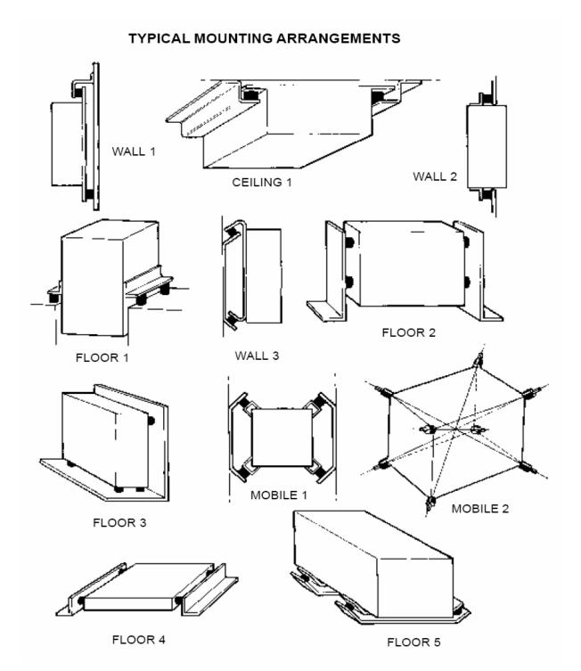
Supporting steel work must be suitably stiffened to minimise flexing and designed to contain spreading forces where an inclined mounting solution is chosen. If in doubt please consult Vibracoustics Ltd directly.
